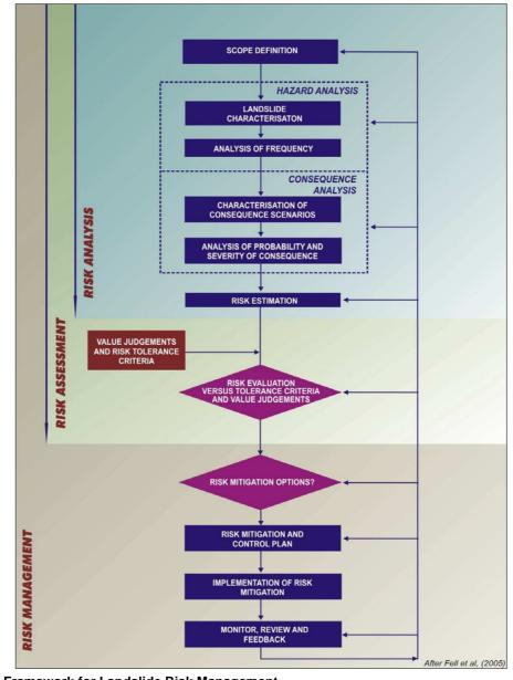
**Figure 5.1. Framework for Landslide Risk Management** Source: Reproduced without amendment from AGS (2007a). Guideline for Landslide Susceptibility, Hazard and Risk Zoning. Australian Geomechanics, Vol 42 No 1 March 2007
