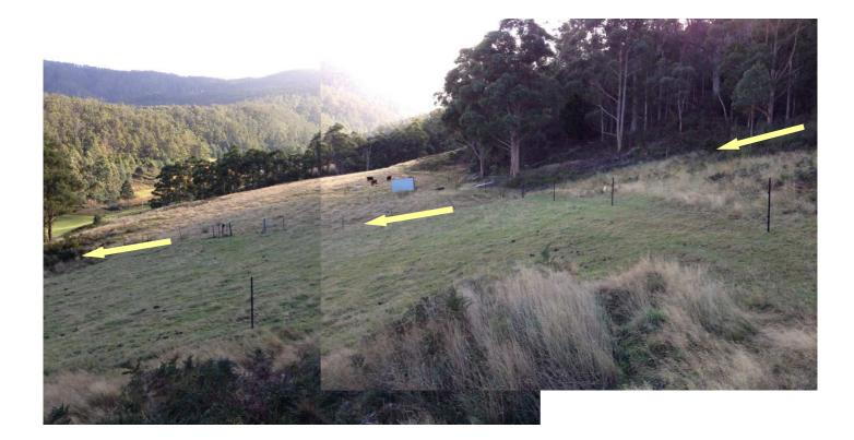
Plates 3 (above) and 4 (below). View north from the house pad. The shallow valley in the middle ground is inferred to be the run-out line (arrowed) of a medium sized shallow translational landslide (probably inactive) which originated on thin colluvial soils on  $25 - 30^{\circ}$  slopes.
