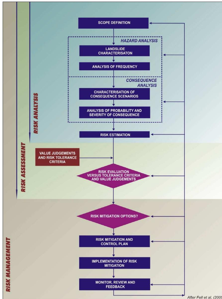
**Figure 5.1. Framework for Landslide Risk Management**
